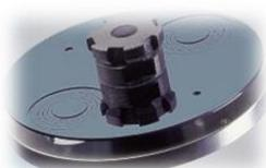
Cu/Constantan disk sensor on Si(X) wafer.
