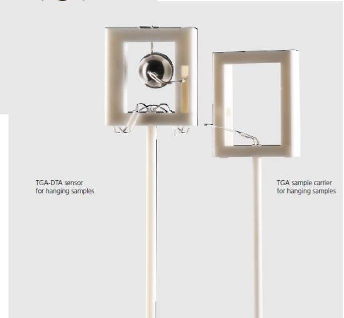
TGA-DTA sensor for hanging samples
