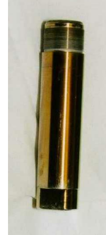
sample holder L = 70 \text{ mm} \varnothing = 15 \text{ mm}
