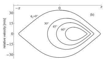
FIG. 1. Transverse and longitudinal properties of the Stark decelerator in its normal mode of operation (s=1). The inset (a) shows the average transverse spring constant as a function of the reduced longitudinal position, relative to the position of the  $\phi_0=0^\circ$  synchronous particle. The inset (b) shows the separatrix in the longitudinal phase space for various phase angles.
