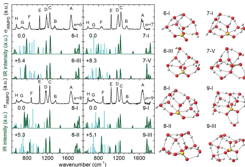
**Figure 4.** Comparison between experimental IRMPD spectra (top black traces) and Gaussian convolution ( $\text{fwhm} = 15 \text{ cm}^{-1}$ ) of the harmonic MP2/6-31+G\* stick spectra (lower green traces) for  $n = 6-9$ . Water librations (blue traces) are not convoluted (see text). Structures and their relative energies (in kJ/mol) are also shown.
