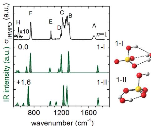
**Figure 2.** Comparison between the experimental IRMPD spectrum (top black trace) and Gaussian convolution (fwhm =  $15\text{ cm}^{-1}$ ) of the harmonic MP2/6-311+G\*\* stick spectra of isomers 1-I and 1-II (lower green traces) for  $n = 1$ . Structures and their relative energies (in  $\text{kJ/mol}$ ) are also reported.
