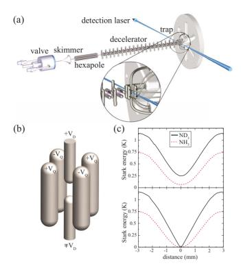
FIG. 2. (Color online) Scheme of the experimental setup, with an expanded view of the IP-type electrostatic trap. The voltages applied to the six cylindrical electrodes are shown (b), together with the resulting potential energies for  $NH_3$  (dashed line) and  $ND_3$  (straight line) along a line in the horizontal symmetry plane for a nonzero (top) and a zero (bottom) electric field at the trap center (c).
