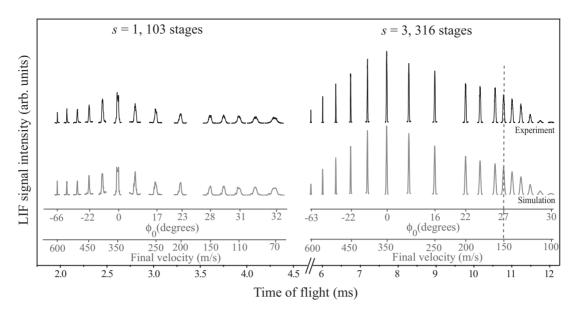
FIG. 4. Time-of-flight profiles of OH radicals that exit the Stark decelerator using the s=1 and 3 mode of operation. The OH radicals are detected after 103 and after 316 electric field stages for s=1 and 3, respectively. The measurements are recorded under otherwise identical conditions, and are shown on the same vertical scale. The beam of OH radicals has a mean initial velocity of 350 m/s. The mean final velocity of the molecules and the phase angle used are indicated for selected profiles.
