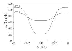
FIG. 9. Natural transverse oscillation frequency  $\omega_y/2\pi$  for an OH  $(X^2\Pi_{3/2}, J=3/2, M_J\Omega=-9/4)$  radical as a function of its phase  $\phi$  in a Stark decelerator, for the operation modes s=1 and 3.
