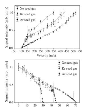
FIG. 7. Maximum signal intensity of decelerated packets of OH radicals as a function of the final velocity (upper panel) and as a function of  $\phi_0$  (lower panel), using a 316 stage decelerator operating at the s=3 mode. Beams of OH radicals with three different initial velocities, produced by seeding in Xe, Kr, or Ar, have been used. The intensities that are obtained from numerical simulations of the experiment are shown as solid lines.
