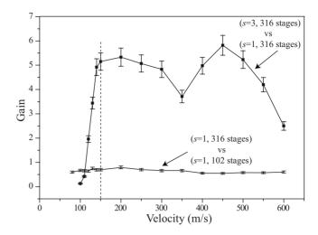
FIG. 6. Lower curve: The ratio of the signal intensity for s=1 operation of a decelerator with 316 vs 103 stages as a function of the final velocity. Upper curve: The ratio of the signal intensity using a 316 stage decelerator operating on the s=3 vs the s=1 mode.
