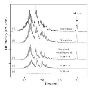
FIG. 3. A measured time-of-flight (TOF) profile of metastable NH molecules observed in a deceleration experiment (a), compared with the outcome of a numerical simulation (b). The molecules are decelerated from 520 m/s to a final velocity of 84 m/s. The contribution of individual  $M_J\Omega$  components to the simulated TOF-profile is shown in the lower part of the figure.
