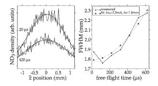
FIG. 8. Determination of the temperature of a packet of  ${}^{15}\text{ND}_3$  molecules trapped in the hexapole trap. On the left, the profile of a packet is shown 20 and 420  $\mu$ s after the trap is turned off (upper and lower trace, respectively). From a fit to a Gaussian line shape the FWHM of the distribution is obtained, as shown as a function of free-flight time (solid line with crosses) on the right-hand side.
