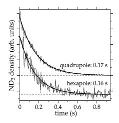
FIG. 9. Density of  ${}^{15}ND_3$  molecules in the quadrupole (upper trace) and the hexapole (lower trace) trap as a function of time that the trap is on.
