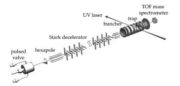
FIG. 5. (Color online) Experimental setup. A pulsed supersonic beam of <sup>15</sup>ND<sub>3</sub> molecules seeded in xenon exits a cooled valve with a velocity of 280 m/s. Ammonia molecules in the low-field seeking hyperfine levels of the  $|J, K\rangle = |1, 1\rangle$  state are focused into the decelerator by a hexapole, decelerated, and then transversally and longitudinally focused into the trap by a hexapole and buncher, respectively. The molecules are detected in a TOF-mass spectrometer.
