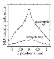
FIG. 6. Density of trapped <sup>15</sup>ND<sub>3</sub> molecules as a function of position in the *z* direction for both the quadrupole trap (upper trace) and the hexapole trap (lower trace), after trapping for about 72 ms.
