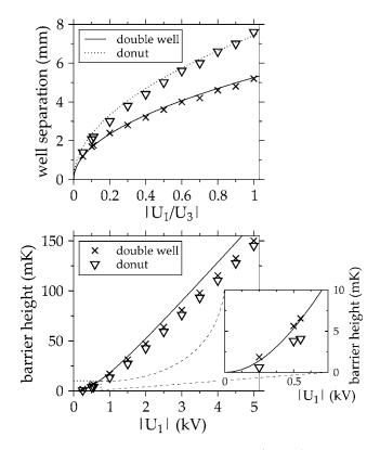
FIG. 4. Well separation as a function of  $|U_1/U_3|$  and barrier height (for <sup>15</sup>ND<sub>3</sub>) as a function of  $|U_1|$  in the ideal double-well (solid line) and donut trap (dotted line). In both graphs the crosses (double-well trap) and triangles (donut trap) show the same quantities obtained from electric field simulations of the actual trap geometry.
