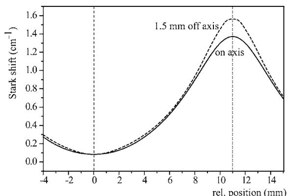
FIG. 4. Stark energy of an OH ( $X^2\Pi_{3/2}$ ,  $J=3/2$ ,  $M_J\Omega=-9/4$ ) radical as a function of its longitudinal position in an electric field stage when the molecule flies on (solid curve) and 1.5 mm away from (dashed curve) the molecular beam axis. The positions of the electrodes are indicated by the vertical dashed lines.
