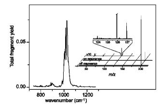
FIG. 3. IRMPD spectrum of  $Cr^+(C_4H_{10}O)_2$ . The inset shows mass spectra taken with the FEL off and on the resonance near 1010 cm<sup>-1</sup>. Observed dissociation channels at m/z=126 and m/z=52 correspond to detachment of one and two ether ligands, respectively. Zooming in on the m/z=126 channel reveals the pattern due to the naturally occurring Cr isotopes, showing the level of detail typically obtainable with FT-ICR mass spectrometry.
