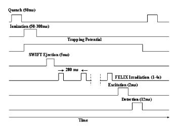
FIG. 4. FT-ICR experimental event sequence used to obtain IRMPD spectra of the fluorene cation.
