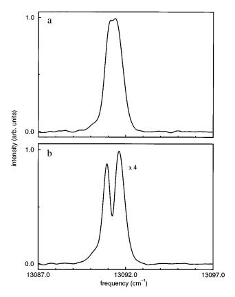
FIG. 3. Fourier transforms of the interferograms presented in Fig. 2. Shown is the spectral intensity distribution at the beginning of the ring-down transient (a) and 2  $\mu$ s later (b). Due to absorption by molecular oxygen, the central part of the spectral profile is observed to decay more rapidly than the wings.
