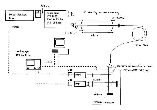
FIG. 1. Schematic view of the experimental setup. Broadband pulsed laser radiation is coupled into an optically stable ring down cavity. The light exiting the cavity is transported via an optical fiber to a Bruker IFS 66v FT spectrometer, with step-scan option. Ring-down transients are recorded as a function of the optical path length difference between the arms of the interferometer on a fast, high resolution digital oscilloscope.
