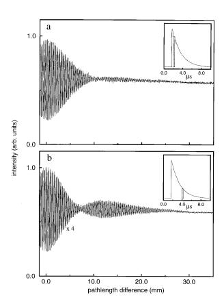
FIG. 2. Interferograms taken at the beginning of the ring down transient (a) and 2  $\mu$ s later (b). The inset shows the ring down transient and the shaded area indicates which part of the transient is used to record the interferograms. A narrow-band light source centered on top of an oxygen absorption line is used.
