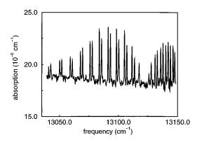
FIG. 6. Absorption spectrum of 15 mbar  $O_2$  in 1050 mbar  $SF_6$  around 763 nm is recorded using pulsed multiplex CRD absorption spectroscopy with the described FT-CRD spectrometer. The spectral structure is due to the atmospheric band, the  $b^1\Sigma_g^+ \leftarrow X^3\Sigma_g^-$  transition, of molecular oxygen.
