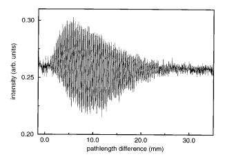
FIG. 4. Normalized interferogram  $I_{\text{norm}}(\Delta,t)$  is obtained by dividing the interferogram shown in Fig. 2(b) by the interferogram shown in Fig. 2(a). This normalized interferogram contains all the required information on the absorption spectrum.
