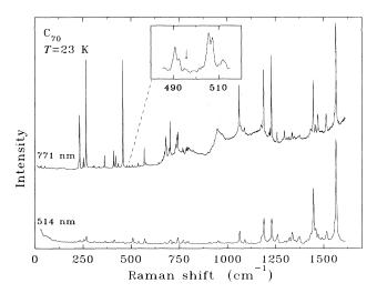
FIG. 1. Unpolarized Raman spectrum of crystalline  $C_{70}$  at T=23 K using 771-nm (upper curve) and 514-nm (lower curve) excitation. The large number of observed modes reflects the relatively low  $D_{5h}$  symmetry of  $C_{70}$ . The inset shows the absence of the 496-cm<sup>-1</sup>  $A_g$  breathing mode of  $C_{60}$  (indicated by the arrow) in the  $C_{70}$  spectra.
