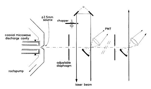
Fig. 1. Scheme of the experimental arrangement.
