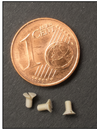
(a) Complete manufacturing a vacuum chamber; \varnothing 264mm, Length: 600mm, 42 flanges; (b) Countersunk screws made of special plastic, M1,6mm; (c) Clamping sleeves of molybdenum
