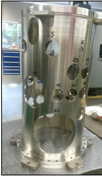
(a) Complete manufacturing a vacuum chamber; \varnothing 264mm, Length: 600mm, 42 flanges; (b) Countersunk screws made of special plastic, M1,6mm; (c) Clamping sleeves of molybdenum
