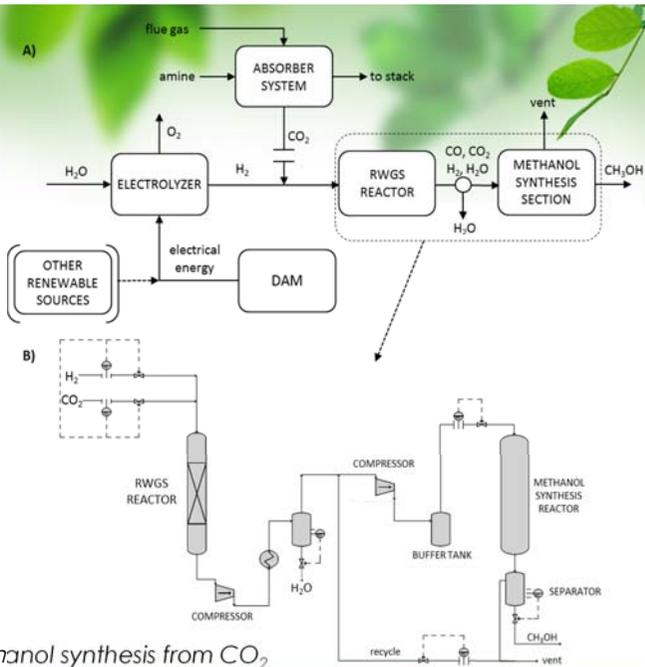
two stages methanol synthesis from CO<sub>2</sub>
