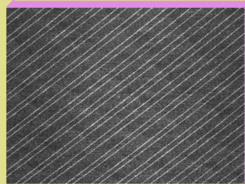
TEM Image: SiO 2 lines (10 nm width) on Si Surface, written by a CNT tip
