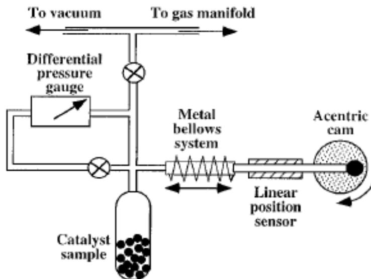
Figure 2. Schematic diagram of frequency response apparatus.
