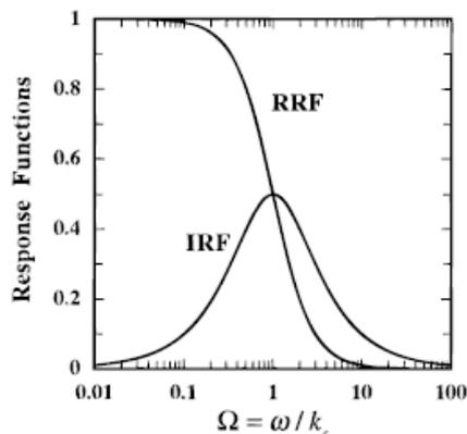
RRF and IRF components for adsorption processes
