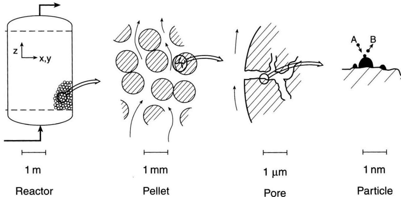
**Figure 7-6** Different size scales in a packed bed catalytic reactor. We must consider the position  $z$  in the bed, the flow around catalyst pellets, diffusion within pores of pellets, and adsorption and reaction on reaction sites. These span distance scales from meters to Angstroms.
