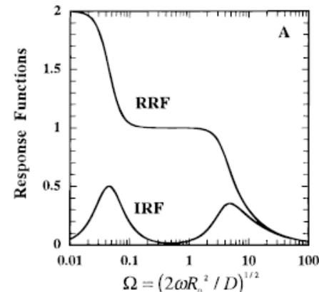
RRF and IRF components for coupled diffusion and adsorption processes
