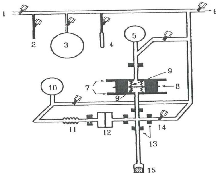
**Figure 1** Frequency response apparatus: 1, vent; 2, gas sorbate inlet; 3, gas sorbate; 4, liquid sorbate; 5 and 10, reference pressure sides; 6, oil diffusion and rotary pumps; 7, electromagnets; 8, moving disc; 9, bellows; 11, flexible glass-metal; 12, differential Baratron; 13, vacuum connectors; 14, vacuum gas tap; 15, zeolite in glass-wool
