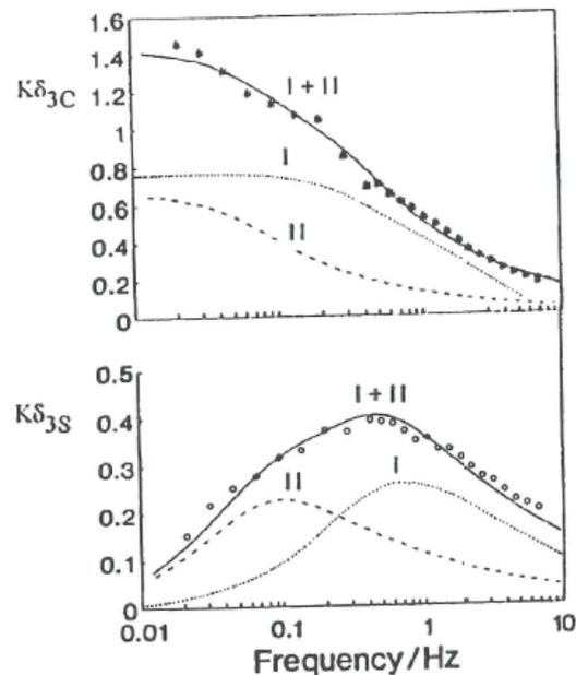
Figure 11 Characteristic functions versus frequency curves for *p*-xylene diffusing in 50 mg of silicalite-1 at 0.431 Torr and 395 K fitted theoretically by lines (I+II) calculated by using Equations (7) and (8) with two diffusion coefficients,  $D_I = 1.8 \times 10^{-11}$  and  $D_{II} = 2.6 \times 10^{-12} \text{ m}^2 \text{ s}^{-1}$
