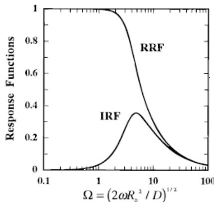
RRF and IRF components for diffusion processes
