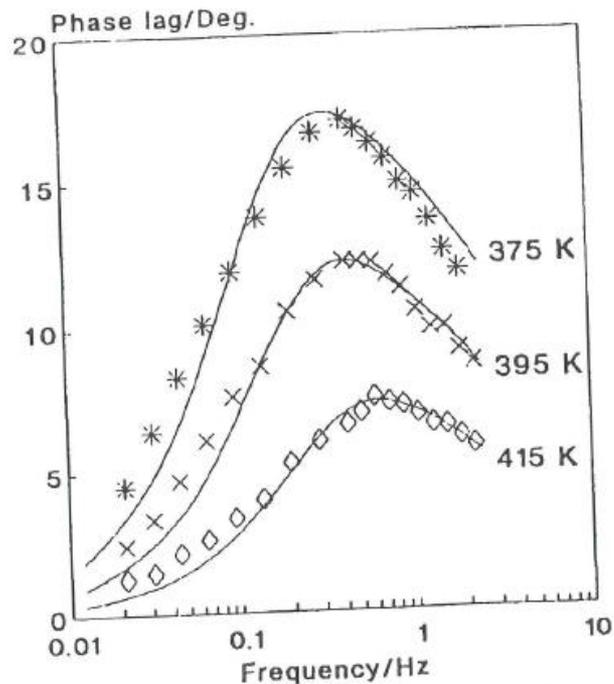
Figure 10 Phase lag versus frequency curves for benzene diffusing in 60 mg of silicalite-1 at 0.862 Torr. Solid lines are theoretically calculated by using Equations (1) and (2)
