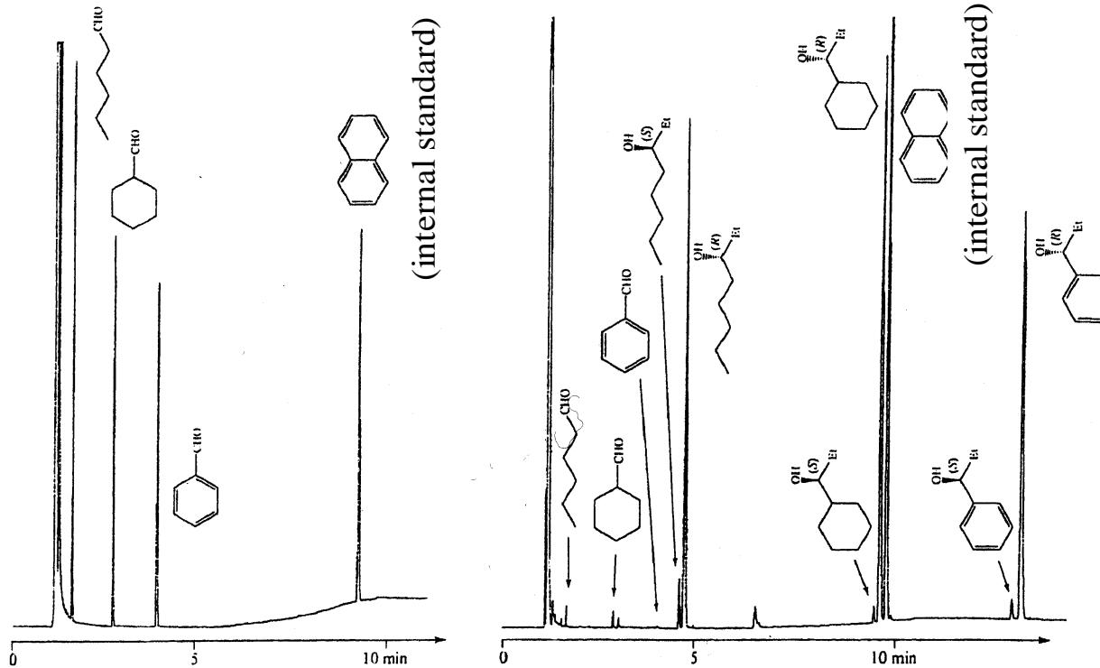
Gas chromatogram of the reaction mixture (left) and GC separation of a representative product mixture obtained by multisubstrate high-throughput screening using (1*R*,2*S*)-*N,N'*-dibutylnorephedrine as the catalyst (right)
