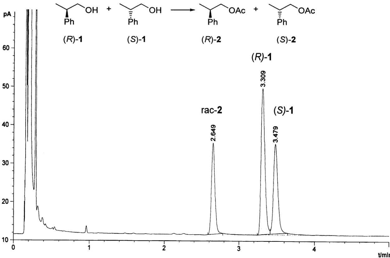
Gas chromatogram of the reaction mixture of the acylation-based kinetic resolution of (R)- and (S)-2-phenyl-1-propanol. 2,3-Di-O-ethyl-6-O-tert.-butyldimethylsilyl- $\beta$ -cyclodextrin was used as CSP
