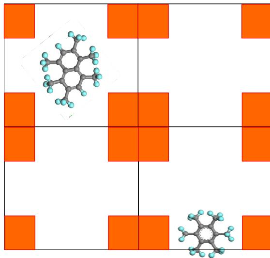
**12-ring window, substituted aromatic hydrocarbons can enter.**
