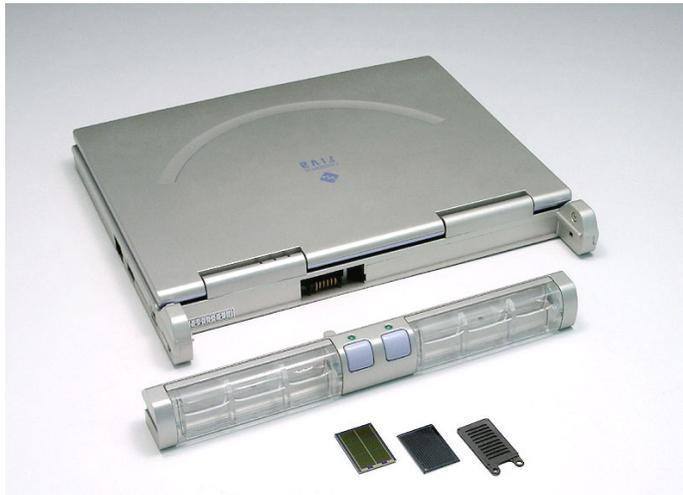
Prototype reformer and PEMFC for a laptop from Casio, about 20 hr of operation.
